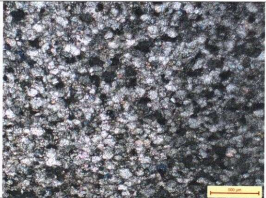
Fig. 3. Photomicrograph shows granular texture of carbonates in dolomite under cross Nicol position (XPL-5X).
