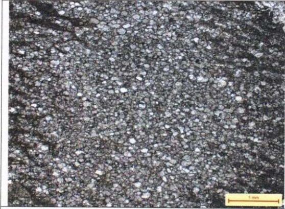
Fig. 2. Photomicrograph shows very fined grained nature of granular carbonates in dolomite under Plane Polarized light (PPL-2.5X).
