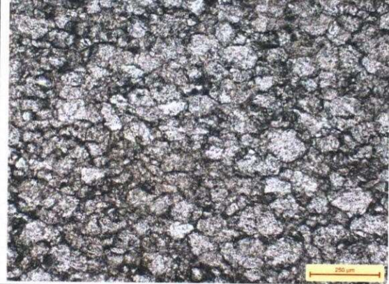
Fig. 4. Photomicrograph showing subhedral carbonate grains with triple junction grain boundaries in Dolomite under Plane Polarized light (XPL-10X).
