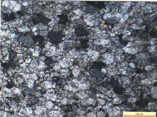
Fig. 5. Photomicrograph of granular texture and triple junction grain boundary in carbonates within dolomite under crossed Nicol position (XPL-10X).
