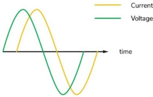
(b) Similarly, when grid is generating Capacitive power, where current leads voltage, SVG detects the phase angle difference and generates a lagging current into the grid making the phase angle of current almost the same as that of voltage on the transformer side, which makes fundamental power factor to unity.
