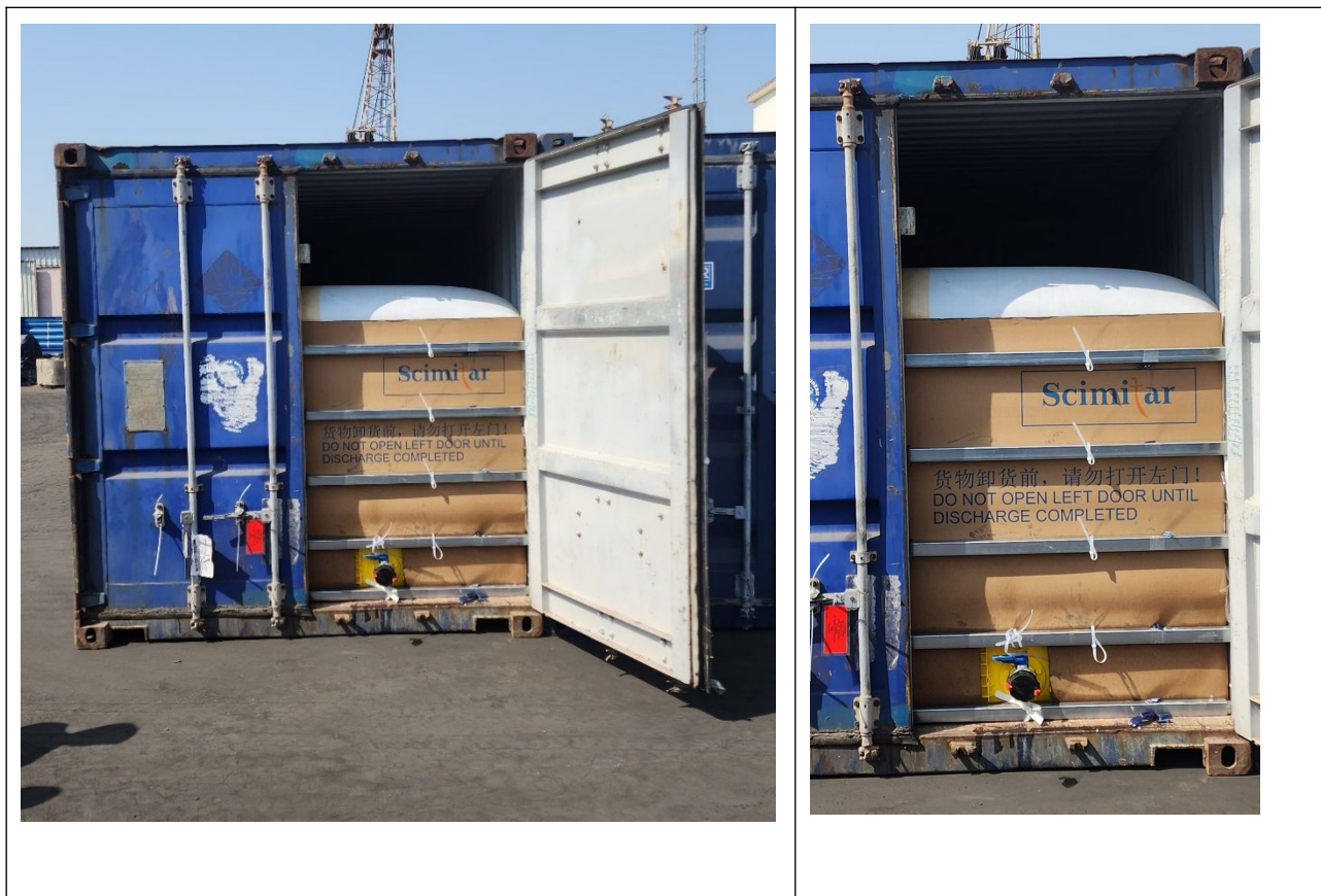
(Pictures of the flexibag containers in the consignment)
