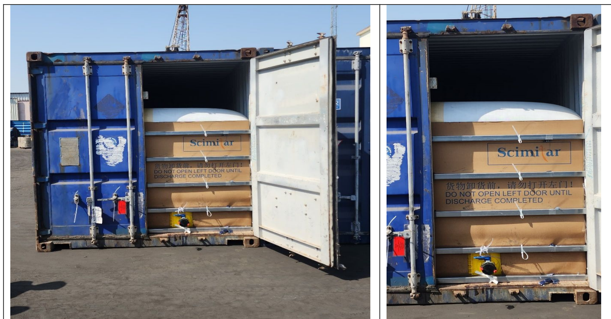
(Pictures of the flexibag containers in the consignment)
