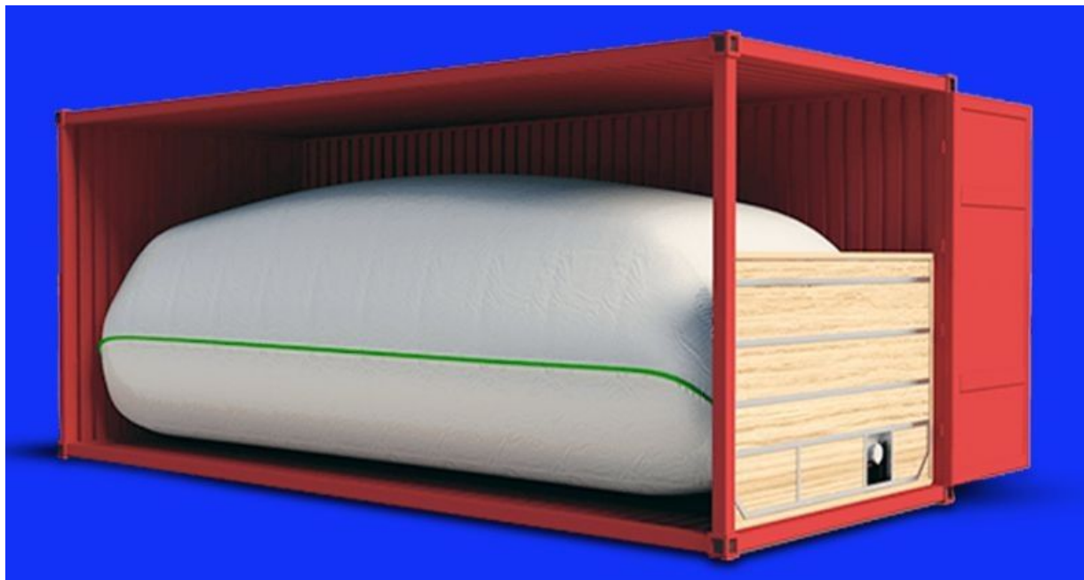
(Graphical representation of a Flexi bag container- picture taken from open source)
